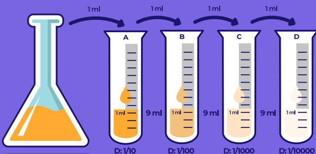
$$F_{d\text{ total}} = F_{d1} \cdot F_{d2} \cdot \dots \cdot F_{dn}$$
